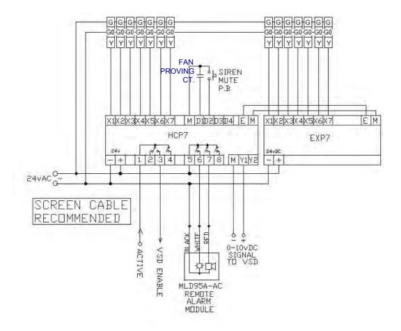
Application Example (4) 12 HEVAC CO sensors , c/w on/off thermostats for temperature control
