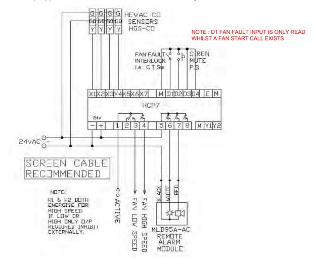
Application Example (2) 4 X HEVAC CO SENSORS & 2 X HEVAC NO2 SENSORS c/w MODULATING VSD OUTPUT
