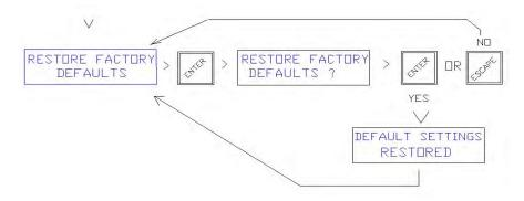
PLEASE NOTE : RESETTING THE CONTROLLER TO FACTORY DEFAULTS SETS THE CONTROLLER TO FULLY CONFORM TO UN-OCCUPIED AS1668.2 MODE SETTINGS USING 8HR TWA FOR ALL OUTPUTS . EX HEVAC SETTINGS ARE SET BEFORE DESPATCH SUCH THAT RELAYS 1 & 3 TO USE CURRENT VALUE AND THE TWA IS ALSO CHANGED TO 1 HR (FROM 8).
